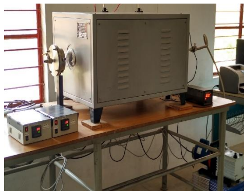
Two-zone tubular furnace attached to a vacuum pump.
